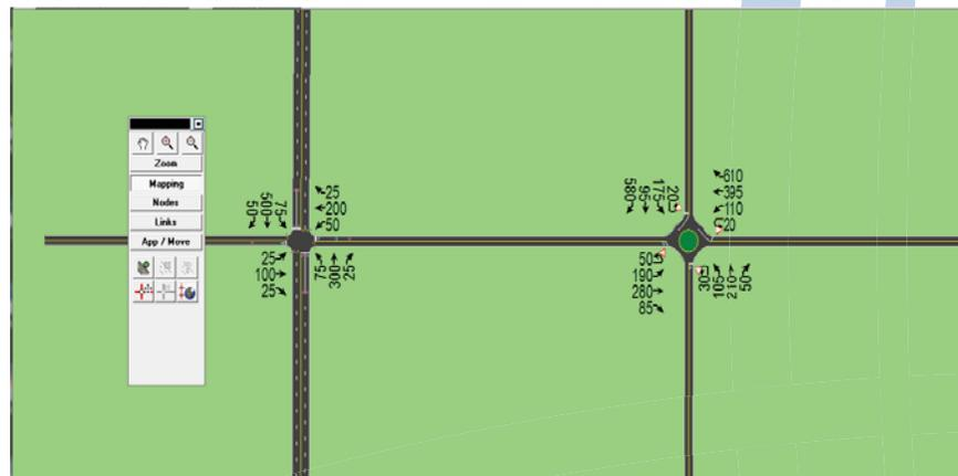
If a more detailed analysis is required, a SimTraffic® model can be developed to provide additional measures of effectiveness. Since SimTraffic® is a microscopic traffic simulation model, it can provide the user a more realistic comparison than a macroscopic model, for example, the overall effect of heavy vehicles upon a traffic stream. Once calibration of the SimTraffic® model has been completed, results on a per-lane basis can be generated.
