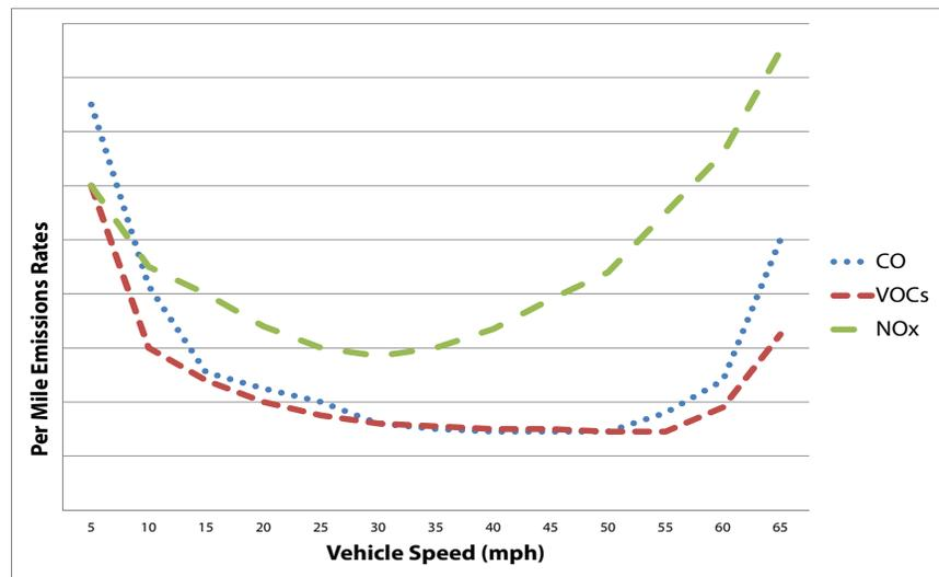
speed and vehicle emissions for three of the most common vehicle emissions. Note that each pollutant has a somewhat different relationship with travel speed.
