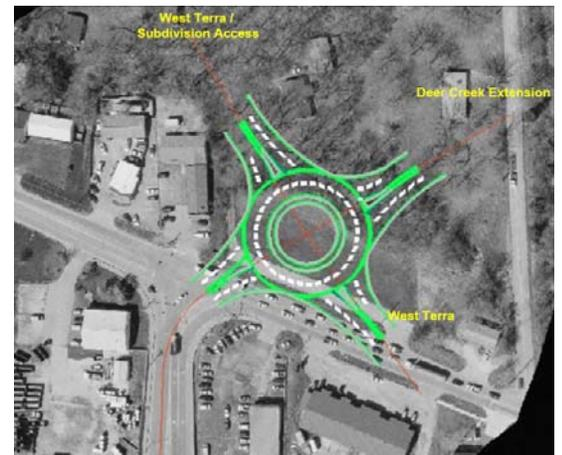
**FIGURE 8 – Revised Four-Leg Roundabout**
