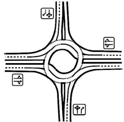
**FIGURE 10 – Traditional Turbo Roundabout Design**
