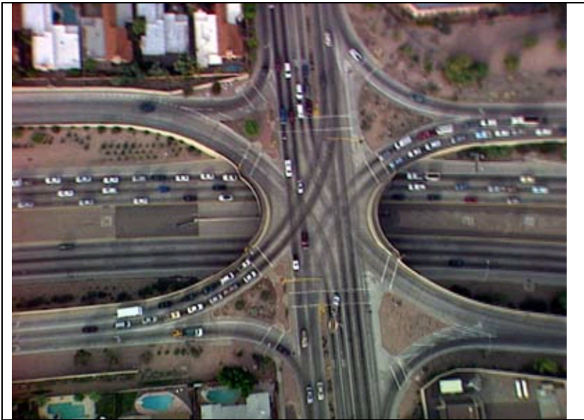
Figure 7-1 Urban Interchange with Overpass
